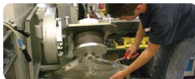
SIEMENS One of 10 000 x-ray tube assemblies being dismantled for re-use of parts.
